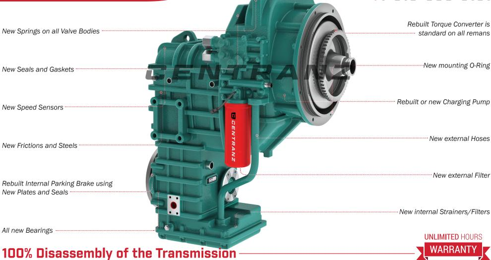
All Transmissions are Dyno Tested and undergo a 5-Step Evaluation: 1) Check Pressures. 2) Check to ensure No Leaks. 3) Check to ensure No Excessive Noise. 4) Function of Solenoid Valves are Evaluated. 5) Function of all Sensors are Tested.
